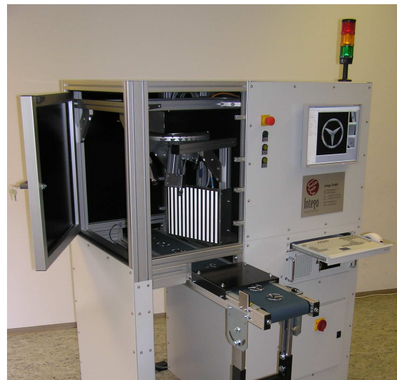
High-gloss surface inspection system with a conveyor belt as buffer.
