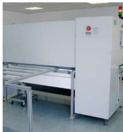
Layup/matrix inspection system for integration into an existing automation (simulated by the roller table).
