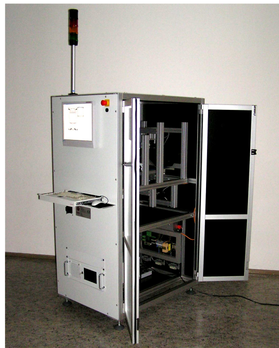
Automatic inspection of transparent parts with OPAL.
