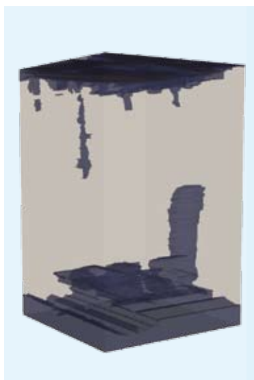
The blue regions are a 3D reconstruction of SiN and SiC impurities in a silicon block due to contaminations in the crystal growth process. These regions shall not be processed further.
