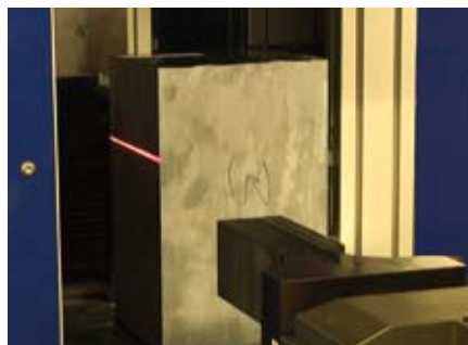
Laser triangulation of the block surface.
