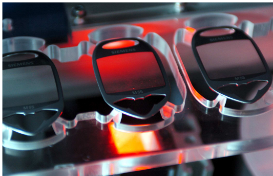
Display lenses of mobile phones have to be fully inspected for production errors.
