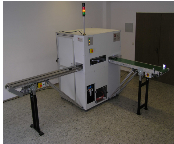
Design variant rotary table with conveyor belt feeding of the parts into the ONYX inspection system.
