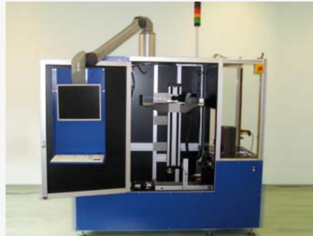
NIR inspection system with manual and automatic operation (top) Detailed NIR image of inclusions in a silicon block (right)
