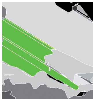
Twin grain recognition: Several parameters for twin grain detection are available. In this case the detected twins are marked green.
